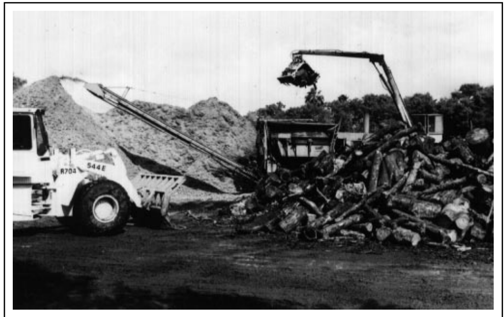
Figure 4.3 Production of Mulch from Logs
