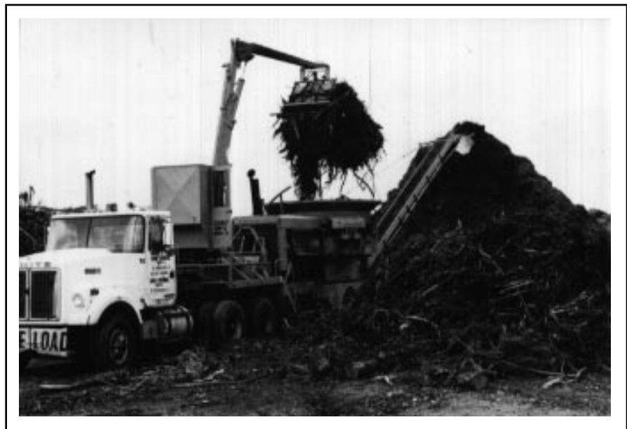
Figure 7.1 Tub Grinder Size-Reducing Yard Trash
