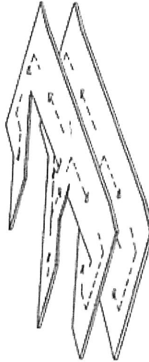
SLOPING FLOORS - CROSS CONNECTED ONE-WAY CIRCULATION
