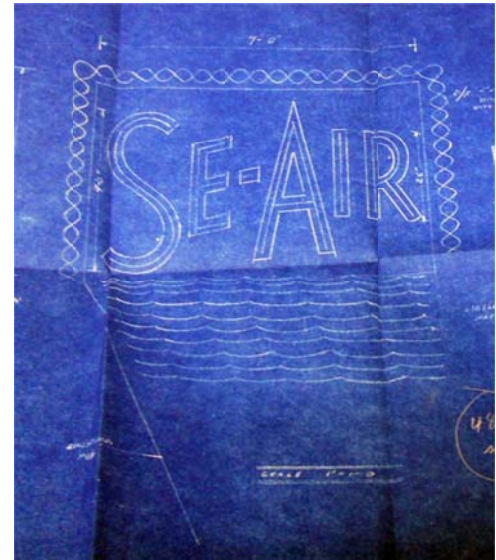
Original blueprint for the neon Se-Air sign, which was affixed to the vertical fin on 9040 Collins Avenue. (Plan courtesy Town of Surfside Building Department Archives.)
