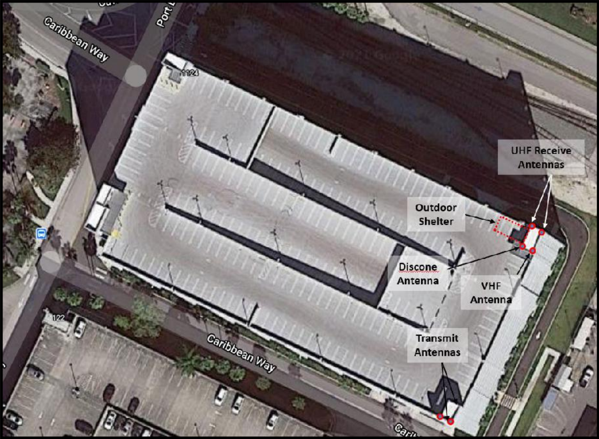
Figure 2-5: Aerial view of Port parking garage
