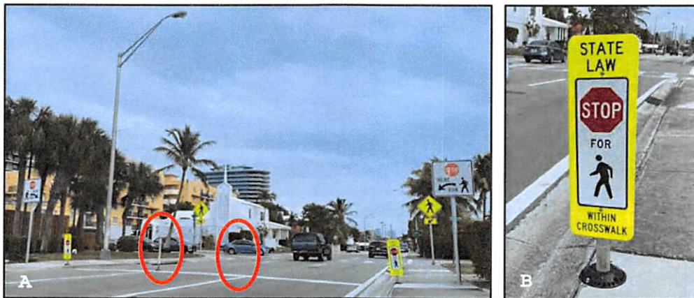
Photograph 5: Missing In-Street Pedestrian Crossing Signs (R1-6a)
