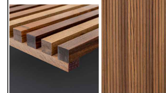
6. WOOD SLATS- WPC (WOOD PLASTIC COMPOSITE) TEAK COLOR Dimensions: 18mm x 160mm x 2.9m Panel Thickness: 21 mm Panel Coverage: 0.36 Panel Weight: About 65 kg/ Acoustic Performance: NRC-0.88 from ISO354. Fire protection performance: Class A from ASTM E84 (US Standard), Class A2 from EN13501 (European Standard)
