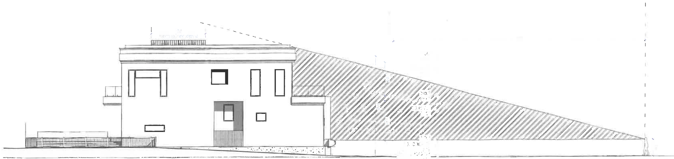
2 LEFT ELEVATION LINE OF SIGHT 1/8" = 1'-0"
